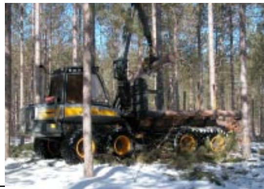
Students visited a variety of logging operations, big and small. Here a forwarder picks up sawlogs for transport to the landing at a larger operation where a red pine forest was being thinned.
