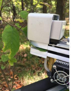
Measuring photosynthesis on leatherwood can be a challenge. The thin leaves that emerge early in the spring tear easily when clamped into the Photosynthesis System (LI-COR 6400, above), so a little creativity is needed to support them when they are inside the chamber -- a stacked tote box and cooler (left).
