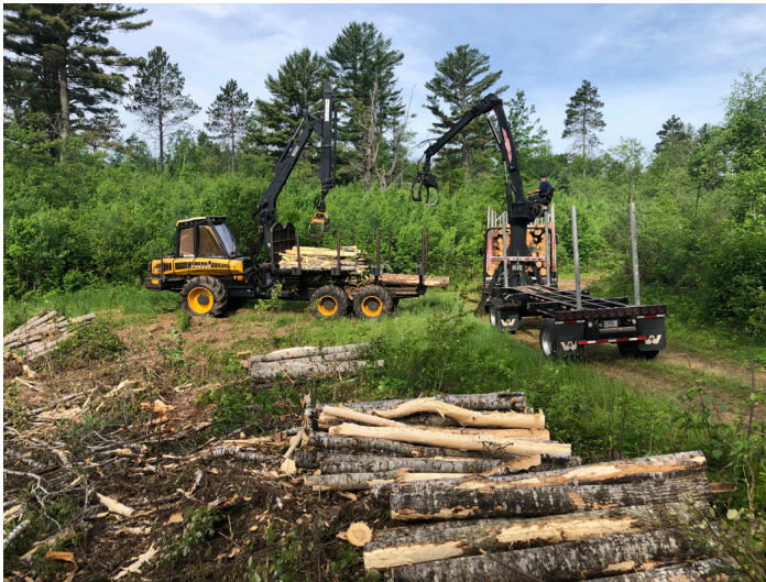
Left: A forwarder and a truck and pup moving timber at a harvest site. Below: A wheeled harvester with a dangle head processor. A four-legged pup for scale. (Photos by Matt Carothers)
