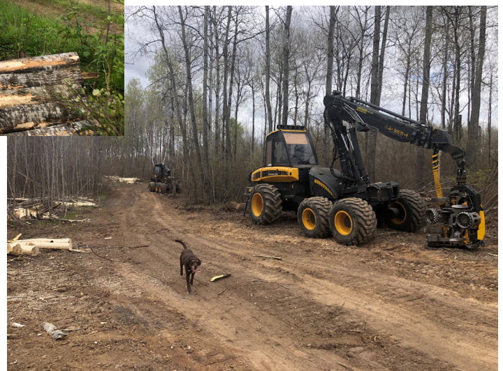
Left: A forwarder and a truck and pup moving timber at a harvest site. Below: A wheeled harvester with a dangle head processor. A four-legged pup for scale. (Photos by Matt Carothers)
